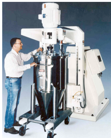
One of the smaller versions of containerized batch mixers, this unit has a 10 cu. Ft. capacity.
