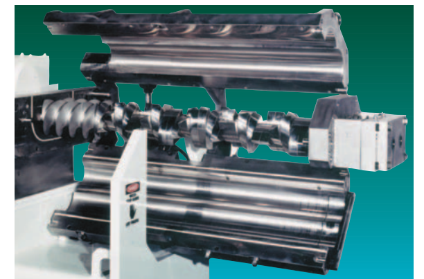
Clam shell design with removable barrel liners reduces operating costs with highly abrasive applications.
